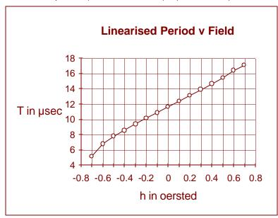
Apart from the droop at -0.7 oersted the linearity has improved considerably. In fact applying the same definition as before the non-linearity between  $\pm 0.5$  oersted has been reduced from 5.5% to 0.7%
