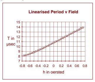
For the miniature sensors a further improvement in linearity and also maximum range can be obtained by making use of the built in overwound coil intended for feedback systems. This can also be used as a simple biasing coil to alter the zero field period of a sensor. Inspection of the graph above suggests that moving the h scale to the right might improve the linearity.
