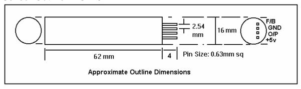
The sensor has been made with a cylindrical form in order to facilitate the overwinding of external feedback coils. Alternatively, it can be readily inserted into a separately fabricated coil on a tubular core.
