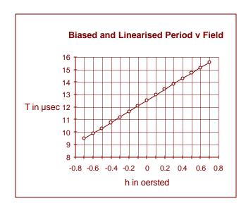
The linear range and linearity can be seen to have improved considerably and applying the same criterion as previously, the non-linearity has been reduced from 4.8% to 0.2% across the increased range of  $\pm 0.7$  oersted.
