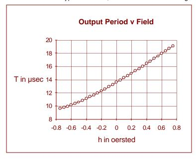
Between  $\pm 0.5$  oersted (  $\pm 50$   $\mu$ tesla ) the non-linearity is about 4.8%
