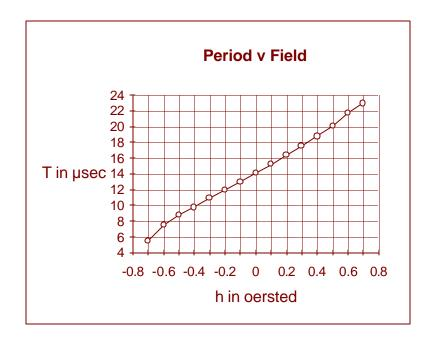
Between  $\pm 0.5$  oersted (  $\pm 50$   $\mu$ tesla ) the non-linearity is about 5.5%.
