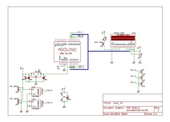
Two sensors can be connected to the circuit, namely to the JP5 and JP6 connectors. The pin (from left to right) are GND, OUT, VCC. The circuit is intended to connect the switch to JP1,
